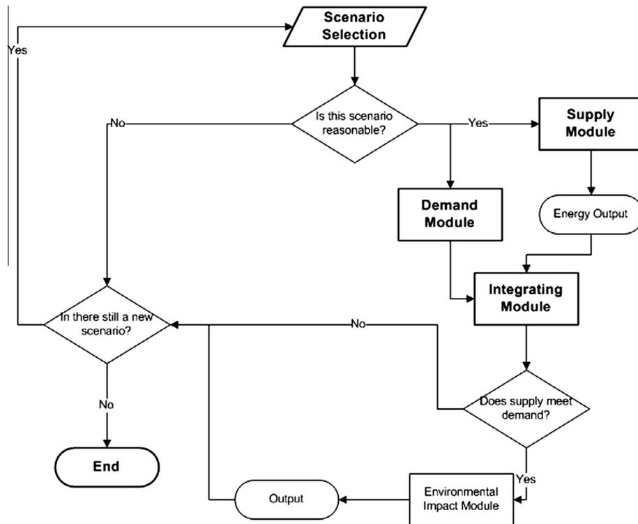
Fig. 2. Simulation procedure of the regional offshore energy analysis model.
