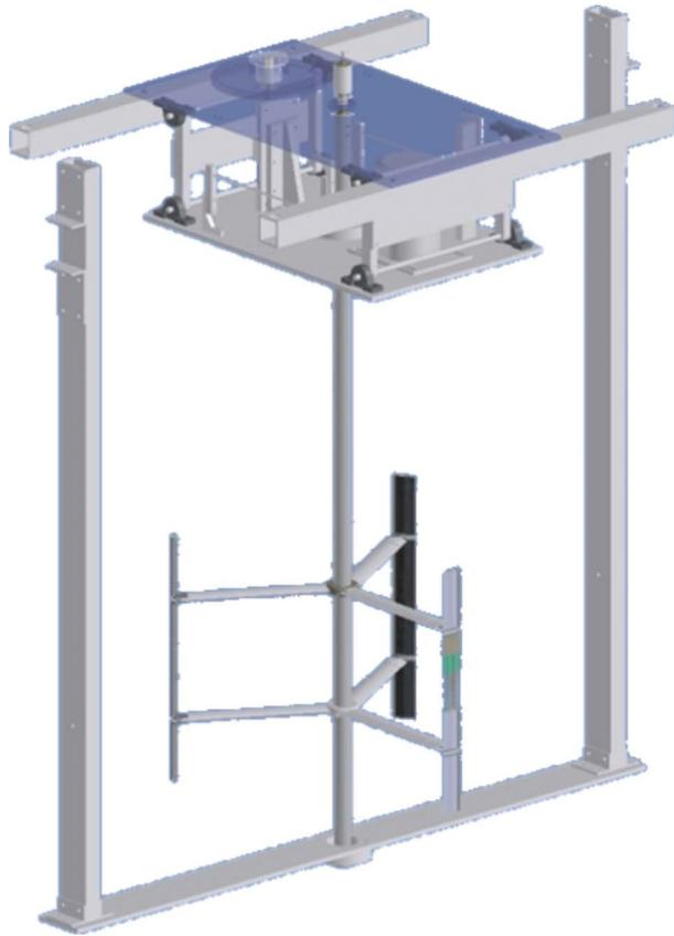
**Fig. 3 An illustration of one of the turbines designed at UBC with the mounting frame**
